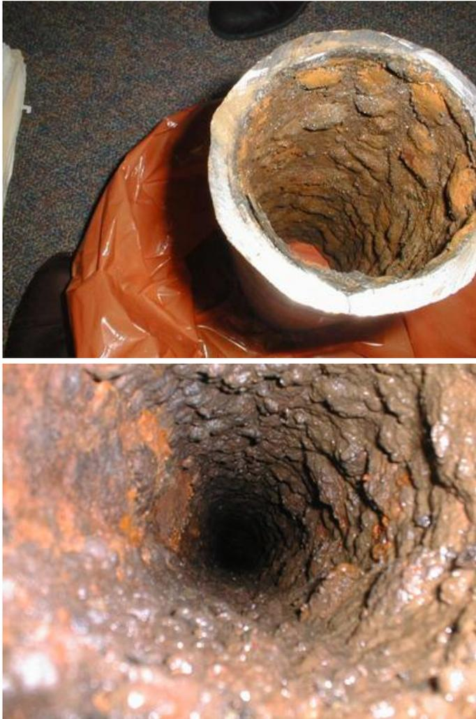
**FIGURE 3. RN PIPING TUBERCLES DUE TO RAW WATER SCALING INCREASE PIPE ROUGHNESS AND REDUCE PIPE DIAMETER**
